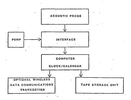
Figure 1: Data Flow Diagram of Automatic Acoustic Groundwater Level Monitoring System.
