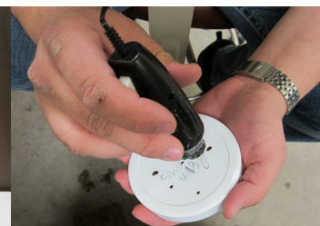
Fig. 5. Using a rotary tool to drill holes into the lid.
