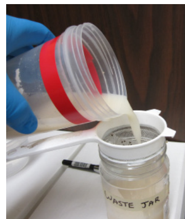
Fig. 9. Straining trap contents.
