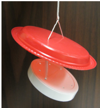
Fig. 6. Example of rain guard attached to lid. Plastic straw spacers between them are optional.
