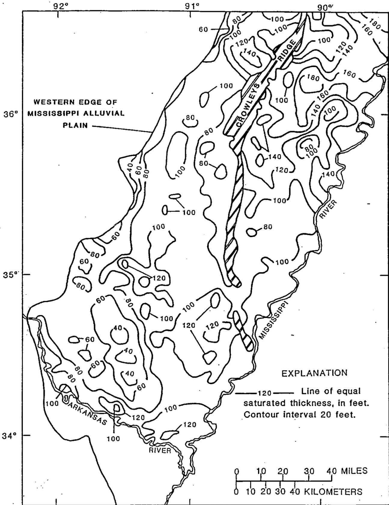
Figure 4.--Saturated thickness of the alluvial aquifer, spring 1982.
