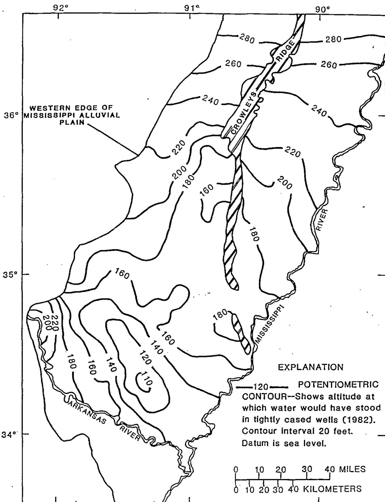
Figure 2.--Potentiometric surface map of the alluvial aquifer, spring 1982.
