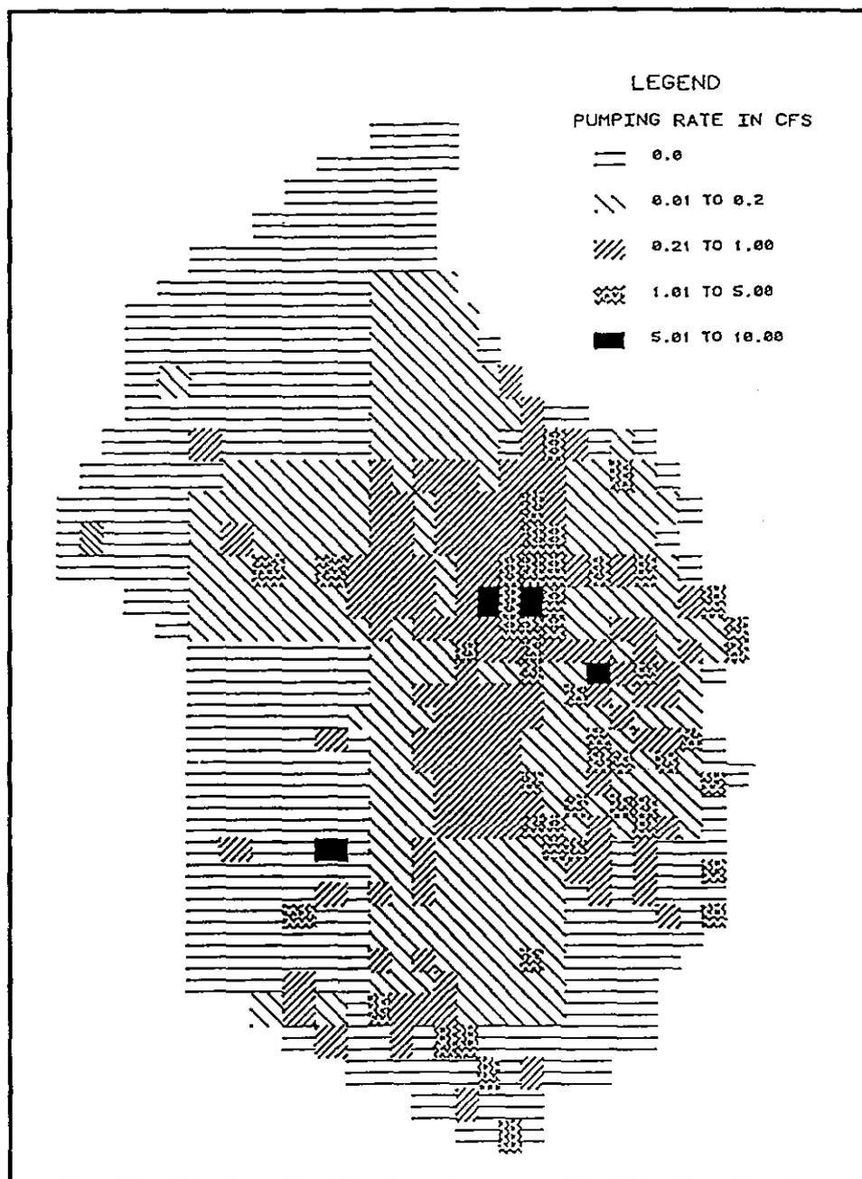
Figure 3. Optimal sustainable pumping rates from lower layer of Salt Lake Valley aquifer system (based on Gharbi, 1991).
