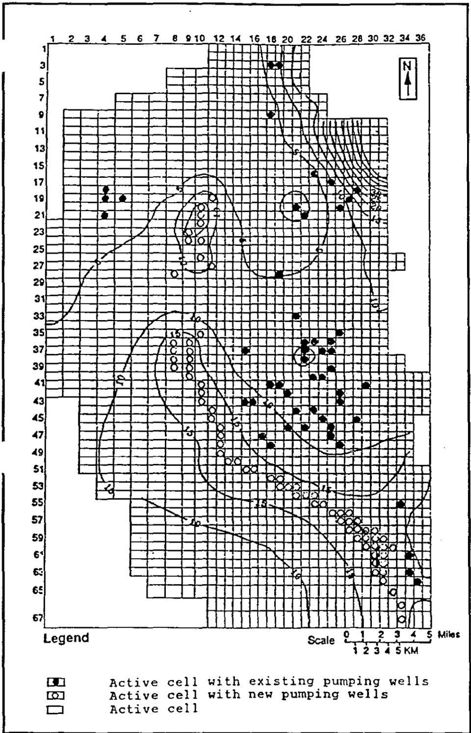
Figure 4. Locations of optimal pumping from Delta Formation, and resulting potentiometric surface elevations, East Shore Area, Utah, (Takahashi, unpublished PhD dissertation, Utah State Univ., 1992).
