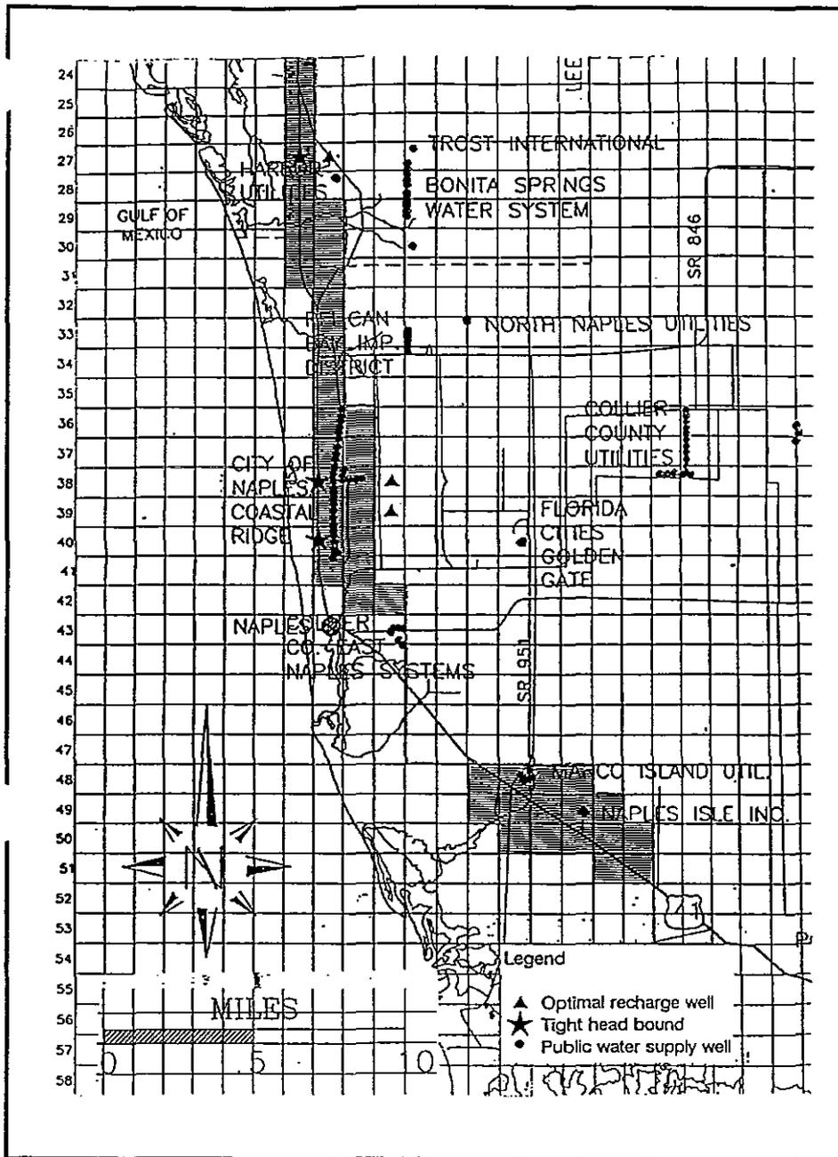
Figure 5. Optimal well locations for minimizing injection needed to prevent salt water intrusion.
