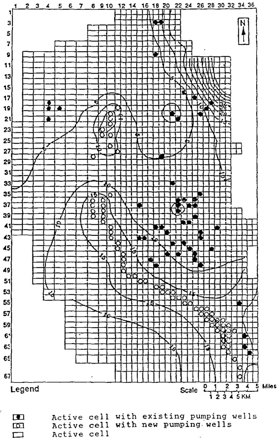
Figure 5. Optimal Well Locations for Minimizing Injection Needed to Prevent Salt Water Intrusion (adapted from Bennett, 1992)
