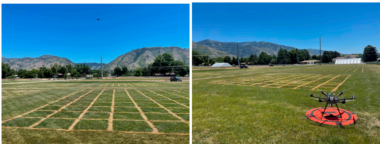
Figure 2. The KBG (1 m × 1 m) plots at the Greenville Farm and the UAV carrying the multispectral sensor during one typical clear day of data collection.
