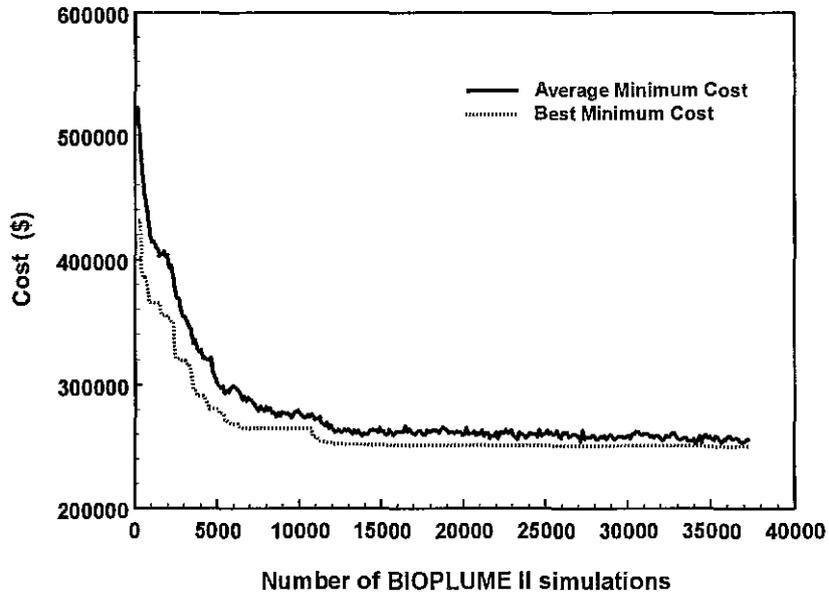
Figure 4. Average minimum cost and best minimum cost vs. number of BIOPLUME II simulations
