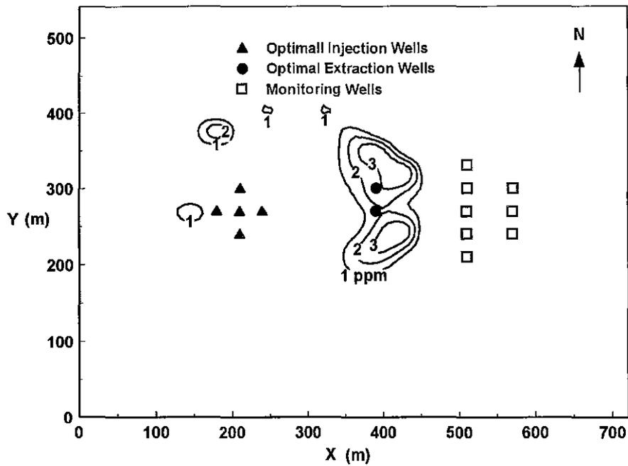
Figure 3. Contaminant plume after 3 years of in-situ bioremediation
