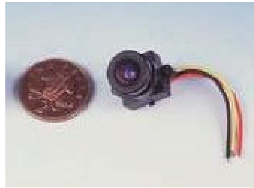
Figure 2: One of the miniature CMOS cameras used on the SNAP-1 MVS.
