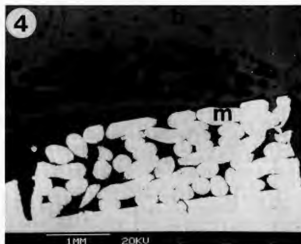
Figures 2 and 3. Bone ingrowth into an acetabular component at three (Fig. 2) and six (Fig. 3) weeks. Figure 4. Bone ingrowth into a femoral component at six weeks. Note the absence of bone ingrowth in the vicinity of the gap at the bone-porous coating interface. B = bone; M = metal fibers.
