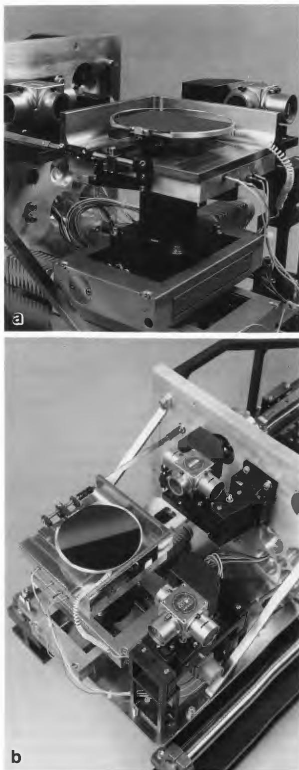
Figure 1. Photographs of the laser interferometer stage. (a) View of the laser interferometer stage unit with a 200mm (4 inch) wafer mounted in the sample position as a scale reference. (b) Interferometer stage unit showing the sample position and interferometry.
