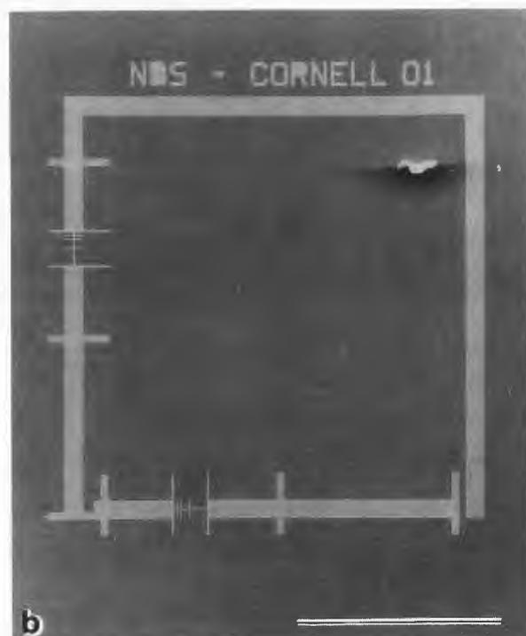
Figure 8. Micrographs of the SEM magnification prototype sample. (a) Low magnification low accelerating voltage. [Accelerating voltage = 1.0 keV; line scale = 500  $\mu\text{m}$ ] (b) Low magnification high accelerating voltage. [Accelerating voltage = 20 keV; line scale = 500  $\mu\text{m}$ ]
