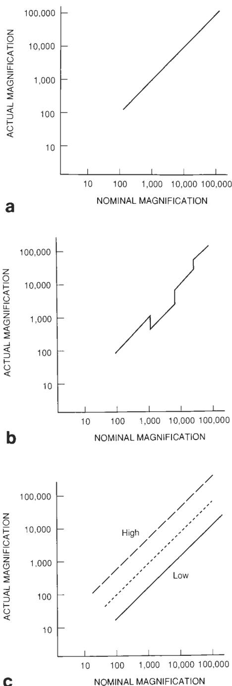
Figure 5. Decade magnification calibration of an SEM. (a) Ideal system where nominal magnification equals actual magnification. (b) Decade system of magnification calibration showing misadjustment between the decades (this has been exaggerated in the Y direction). (c) Proper decade calibration where the gain of the overall system can be adjusted higher or lower to achieve the proper magnification (central line).
