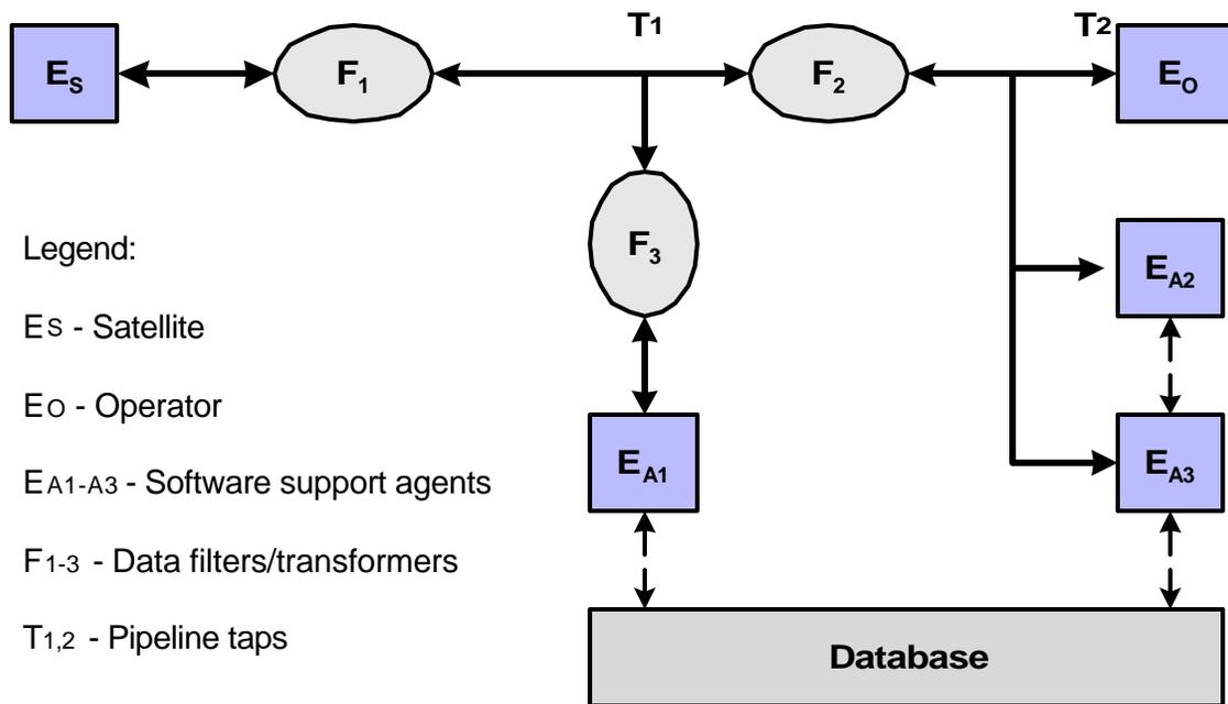
Figure 2 – Diagram of data pipeline used during Opal communication.
