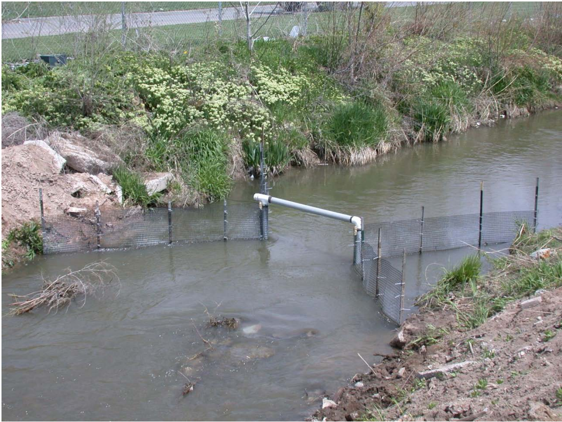
Figure 2. Photo of the “pass through” design interrogation system set up in Battle Creek. All interrogation systems were set up similar to this except the Provo River, which were anchored to the bottom on all four corners.
