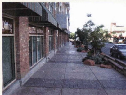
This section of Main Street portrays an appropriate treatment of sidewalk and planting strips in an urban
