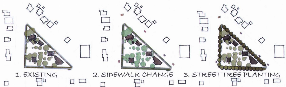
Fig. 20 This series of conceptual drawings outlines (1) the existing condition of many planting strips, (2) the approach of removing sidewalks that are integrated with curbs, setting them back six to twelve feet, and then (3) planting street trees.
