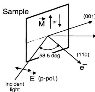
FIG. 2. Experimental geometry used in spin-polarized photoemission measurements.
