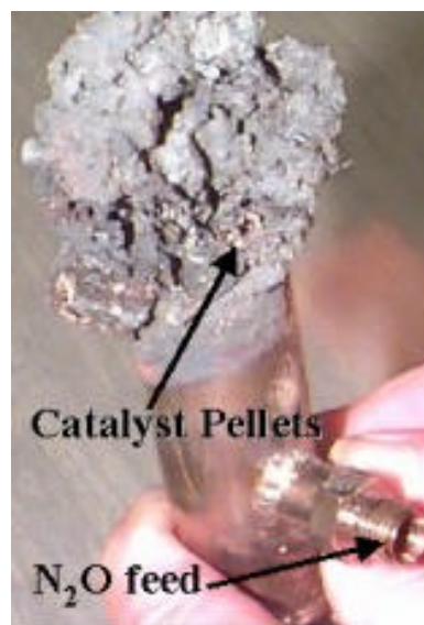
Figure 8. Test design after firing: a) Stainless steel pipe is melted with iron catalyst and MICROPORE thermal insulation; b) Alumina pellets coated by catalyst have survived the heat.
