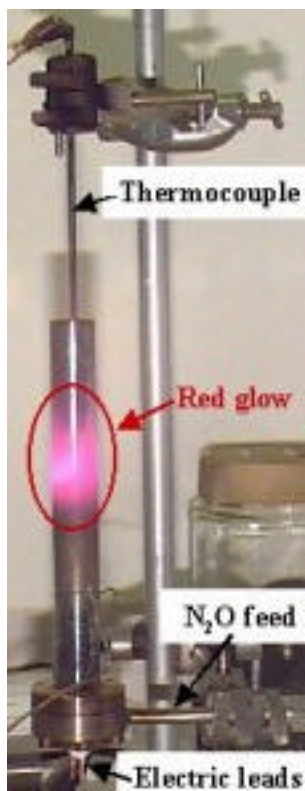
Figure 6. Self-sustaining nitrous oxide decomposition on LCH 212 hydrazine catalyst. The electric leads have been disconnected from power supply after “ignition”. No electric power is applied.
