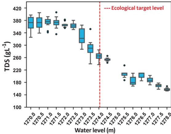
**Figure 1:** Total dissolved solids (TDS) vs. Lake Urmia level from 1977–2017. Boxes depict the 25<sup>th</sup>, 50<sup>th</sup>, and 75<sup>th</sup> percentiles of measurements between indicated lake level and next highest lake level. Bars and diamonds show the range of TDS data and outliers. For comparison, the TDS of seawater is near 35 g L<sup>-1</sup>.
