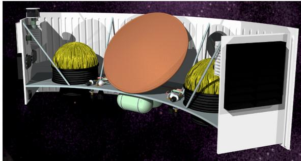
Figure 6 shows an artist's concept of the probe carrier. The object in the center is an example of one large probe. The tanks are to either side of the probe. The tank below the probe is a pressurant tank for the bi-propellant system. The end structural pieces contain louvers for thermal control and spacecraft electronics. The white "corrugated" structure behind the probe is the backside of the solar array structure.
