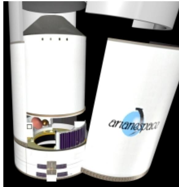
Figure 8 shows a rough layout of the Ariane 5 during a micromission launch. The artist's concept shows the upper stage and fairing as the fairing begins to fall away. The lower part contains the ASAP5 structure with secondary micromission mounted on top. The two primary payload communications satellites are stacked on top. This is preliminary artwork from a micromission animation that will be finished in the fall of 1999.
