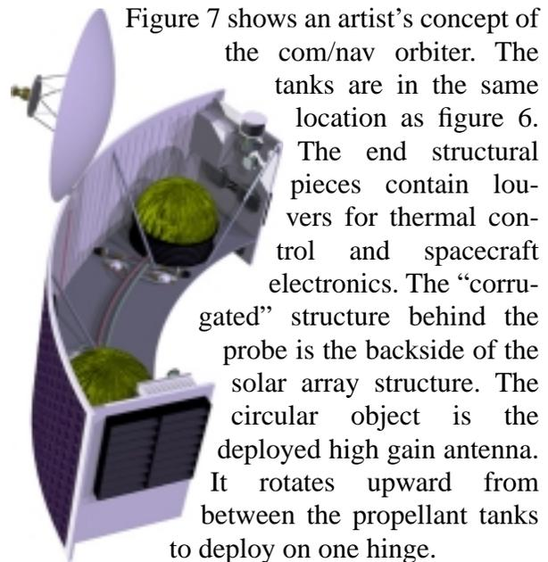
Figure 7 shows an artist's concept of the com/nav orbiter. The tanks are in the same location as figure 6. The end structural pieces contain louvers for thermal control and spacecraft electronics. The "corrugated" structure behind the probe is the backside of the solar array structure. The circular object is the deployed high gain antenna. It rotates upward from between the propellant tanks to deploy on one hinge.
