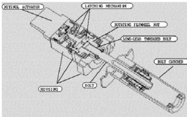
**Figure 8: FASSN Cross-Section**
