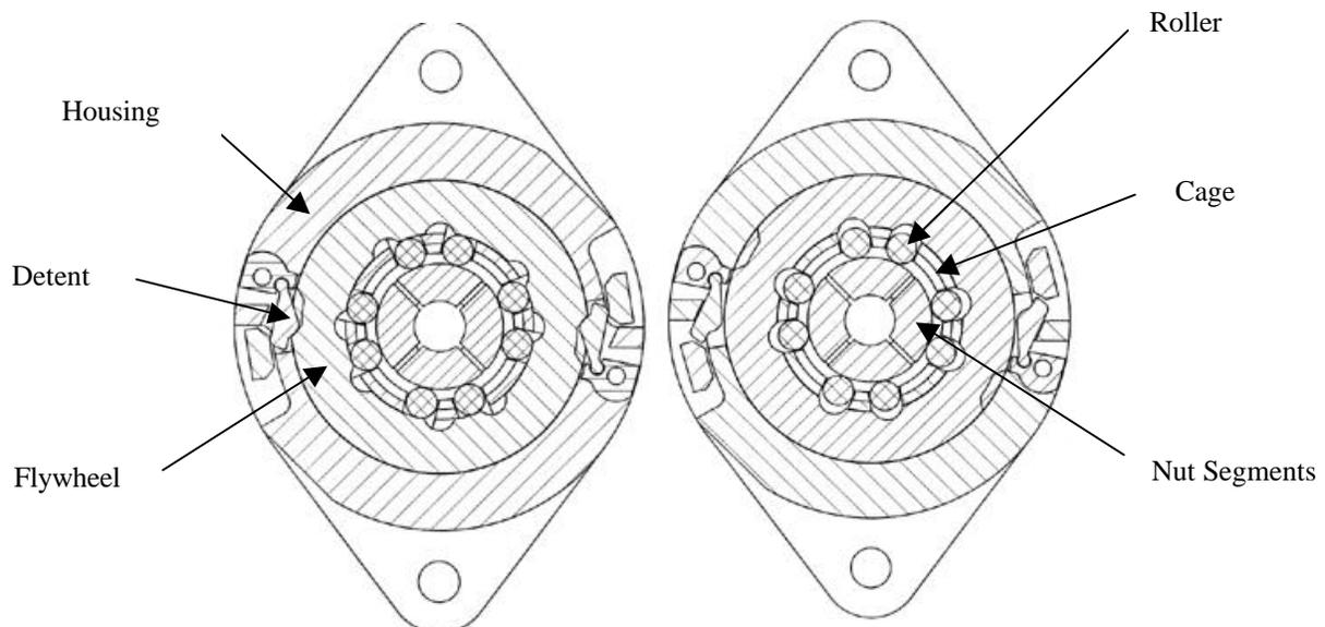
**Figure 3: Qwknut in latched and released conditions respectively**
