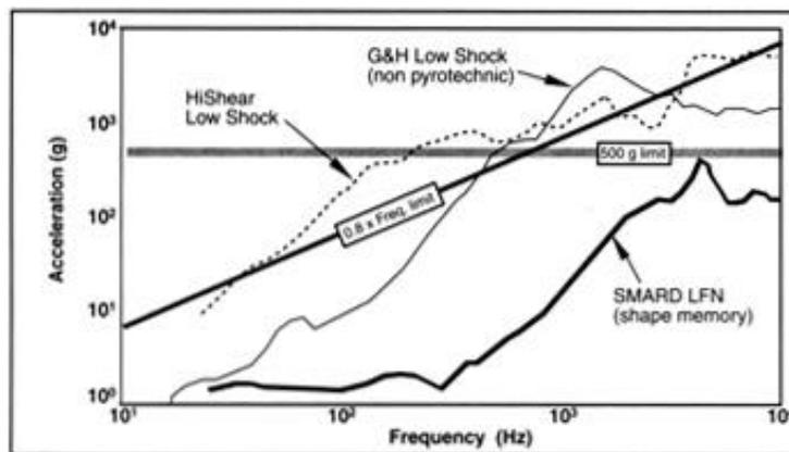
**Figure 2: LFN Shock Response, 3000 lbf Release**
