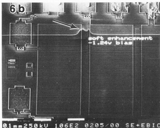
Figure 6: Y-modulated EBIC signals, indicated by arrows, on capacitors (450Å), showing different locations of the defects in the oxide: (a) within the field of the capacitor, (b) at the LOCOS edge of the capacitor.
