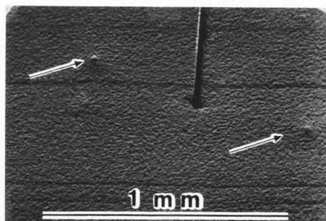
Figure 5: EBIC spots in Y-modulation in capacitors ( $90\text{\AA}$  oxide) as observed in accumulation or depletion.
