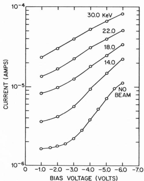
Figure 4: Electron beam induced current (EBIC) distributions as a function of negative bias at various electron beam energies.
