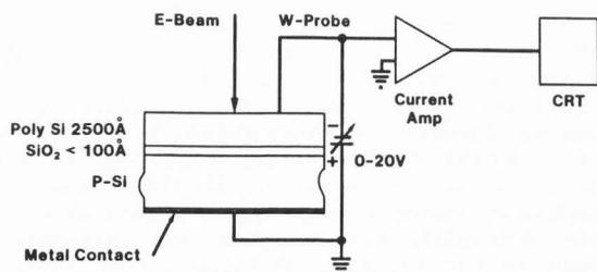
Figure 3: Experimental arrangement for EBIC imaging of thin MOS oxide defects.
