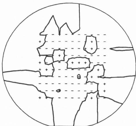
Figure 2: Contour map of breakdown voltage data for thin oxide capacitor on a 4-inch Si wafer. (+) denotes site of defective capacitor.
