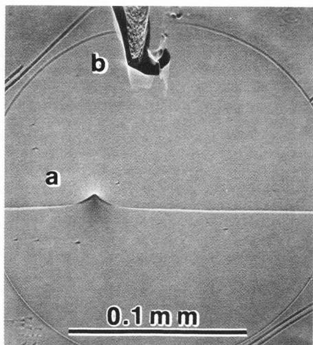
Figure 1: Circular capacitor of  $3.2\text{mm}^2$  area with EBIC spot (a) and probe contact (b) in y-modulation mode.
