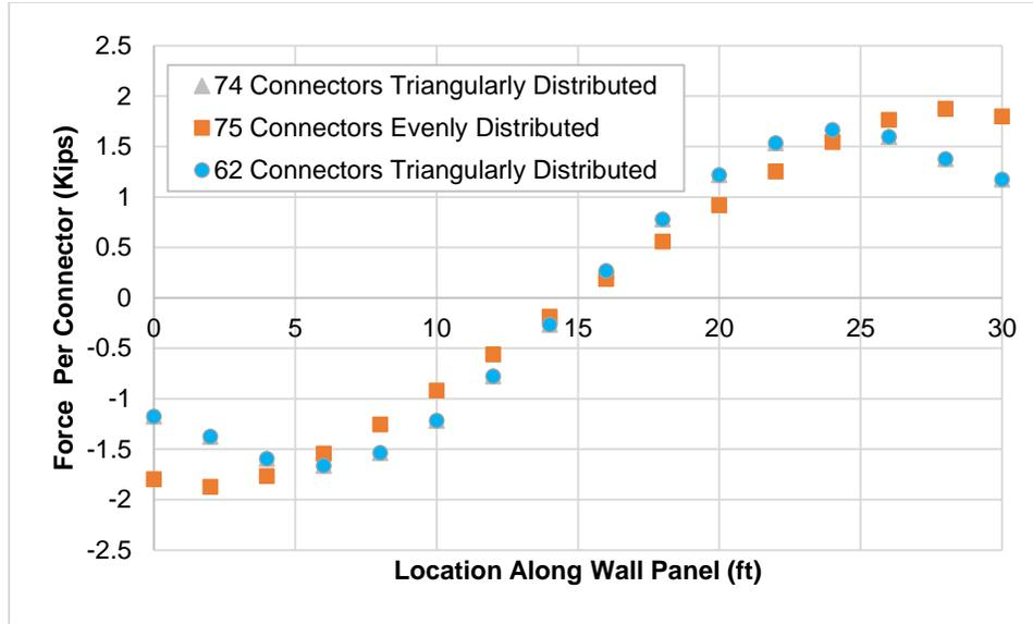
Figure 11 – Force per Connector for Different Connector Distributions
