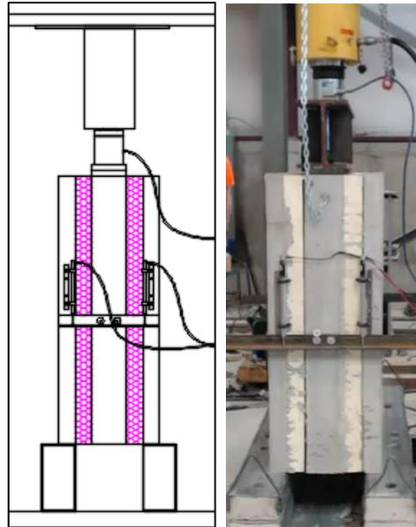
*Figure 2 – Push-off Test Setup*
