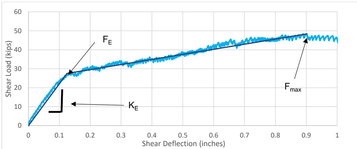
*Figure 5 Determination of Elastic Load and Stiffness*
