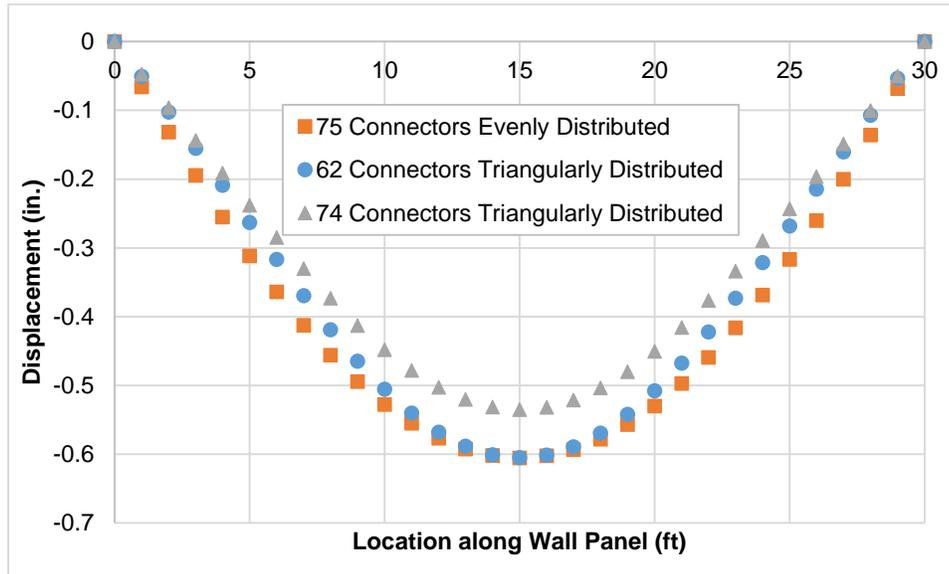
Figure 7 – Deflection Comparison with Different Connector Distributions
