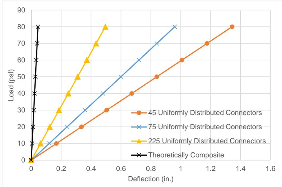
Figure 8- Example Elastic Load versus Deformation Relationship for Various levels of Shear Connector Intensities
