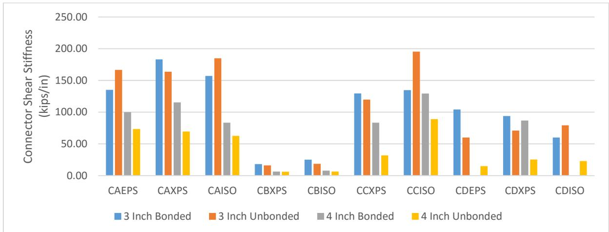
*Figure 7 - Elastic Stiffness ( $K_E$ ) across Specimens (per connector)*
