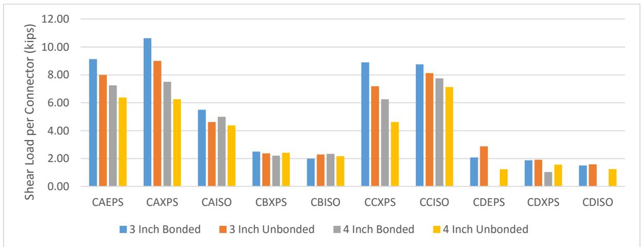
*Figure 6 – Elastic Limit ( $F_E$ ) Comparison (per connector)*
