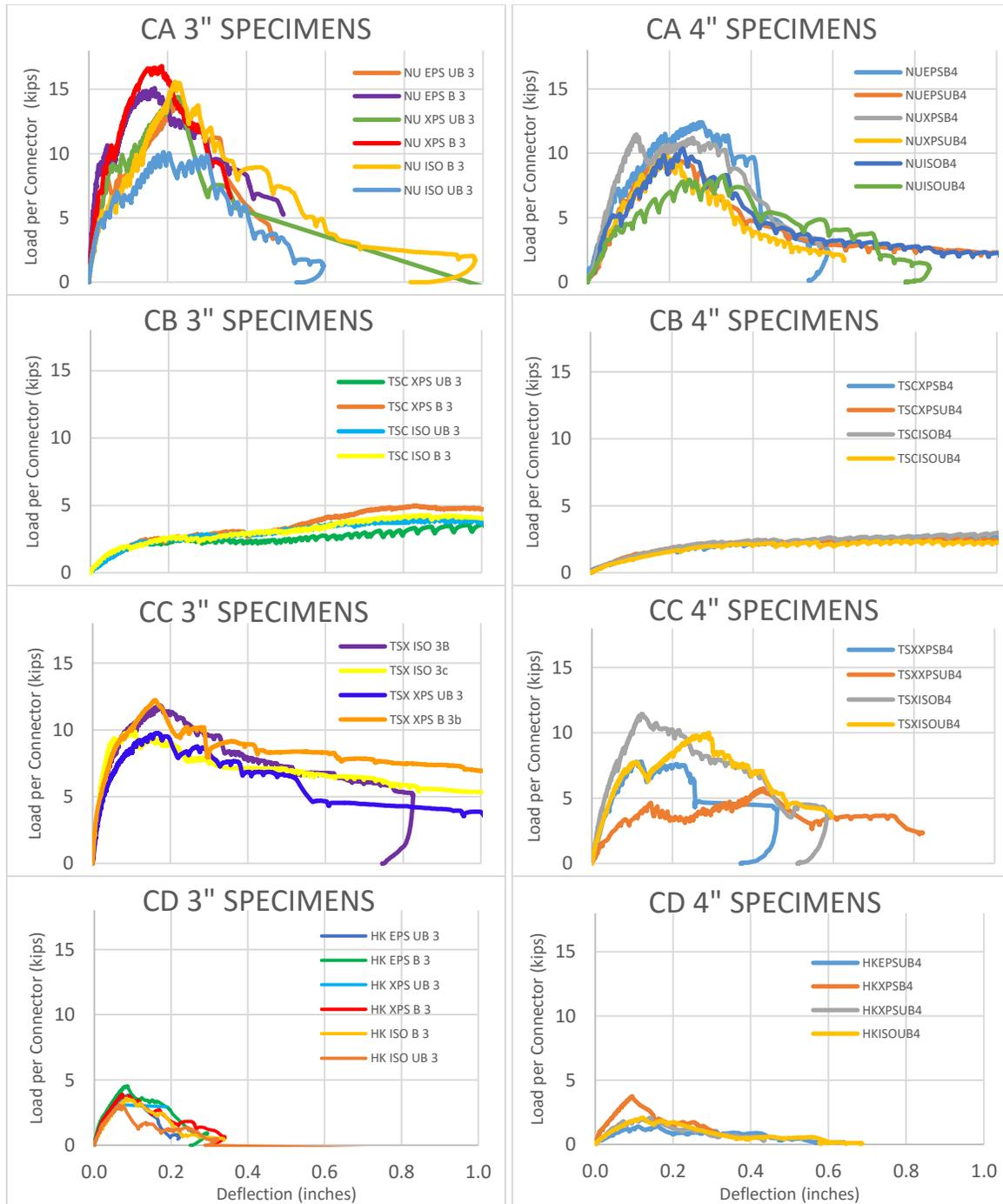
Figure 3 – Load versus Deformation for all shear connectors in this study
