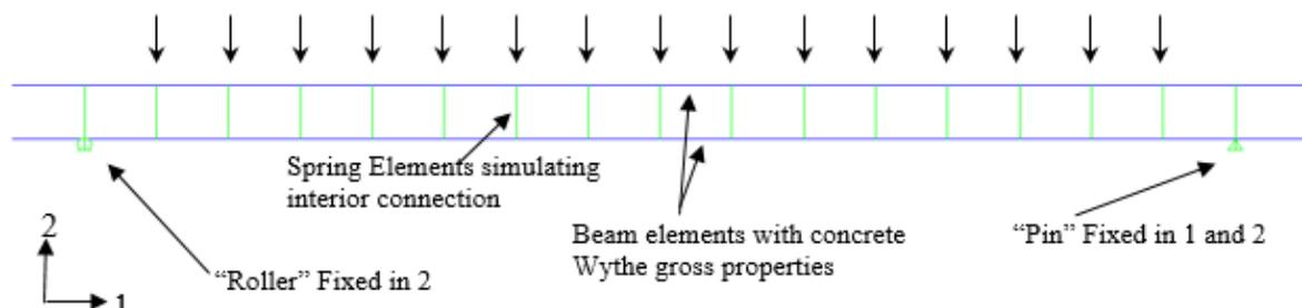
Figure 5 Beam and Spring Model used to model Naito 2009 Full Scale Specimens
