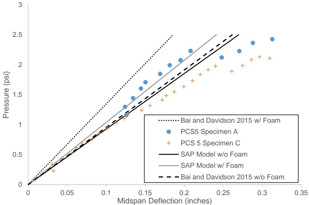
Figure 6 Deflection and Resistance Comparisons in Elastic Range for PCS5 Specimens from Naito et al (2011)
