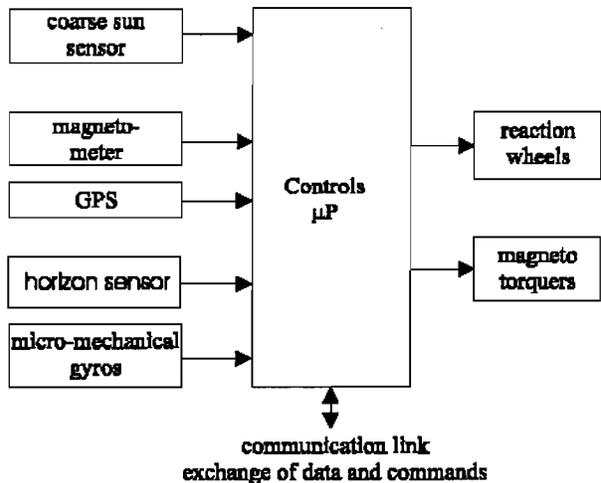
**Figure 8: GNC block diagram**
