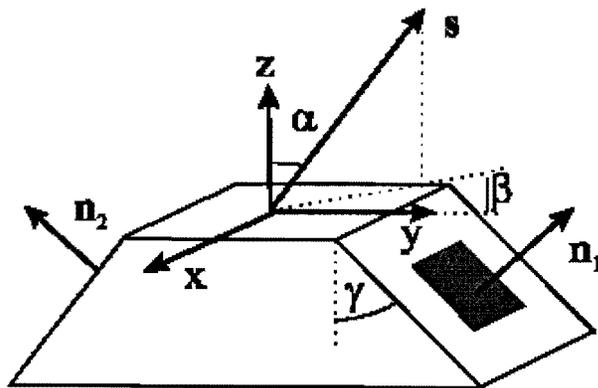
Figure 9: GNC Sun Sensor Concept
