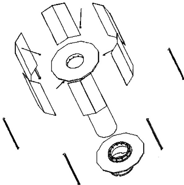
**Figure 5: UASat Preliminary Structure Design (Exploded View)**
