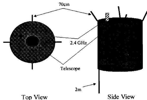
**Figure 6: UASat Antenna Locations**
