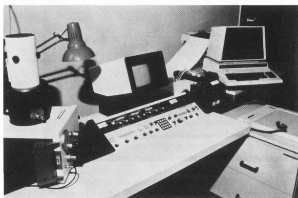
Fig. 4. Experimental set up showing the Stereoscan 100 on the left and the digitizer with the CBM computer on the right side.
