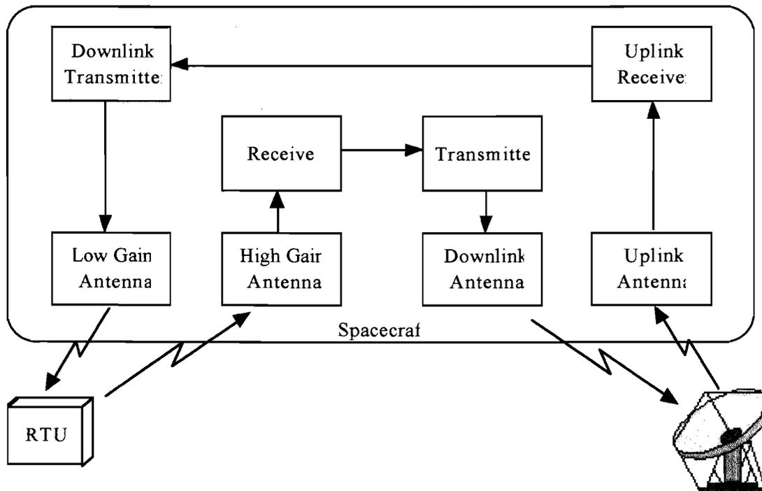
Figure 1: Analog Bentpipe Communications Concept
