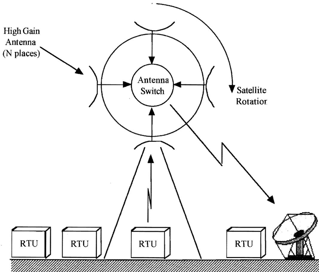
Figure 2: Scanning High Gain Antenna Concept (Spin Stabilized Option)
