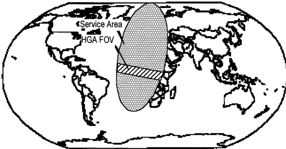
Figure 3: Satellite Service Area of Field of View of the Scanning High Gain Antenna
