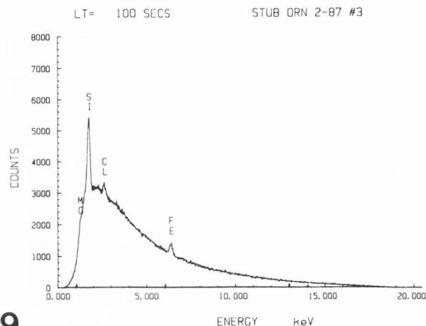
Fig. 9. Representative spectrum of vinclozolin particles found on stubs. Note presence of chlorine.
