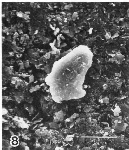
Fig. 8. Sharp-edged, agglomerated particles found on stubs adjacent to *Rhododendron* leaf when exposed to vinclozolin smoke. Bar = 5  $\mu$ m.
