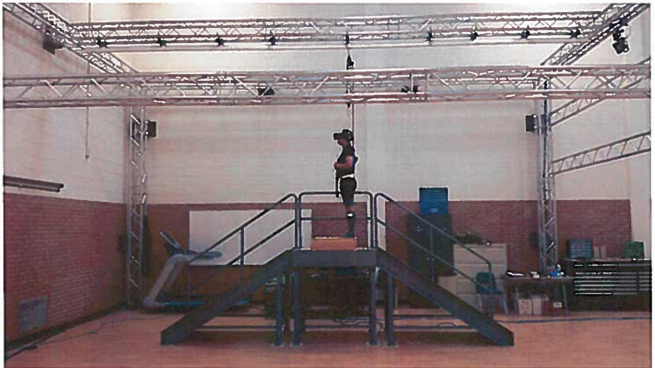
Figure 1: Image of the experimental setup illustrating a participant wearing the harness tethered to a freely moving track above the stairs to prevent falls.
