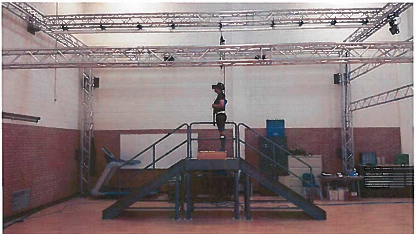
Figure 1: Image of the experimental setup illustrating a participant wearing the harness tethered to a freely moving track above the stairs to prevent falls.
