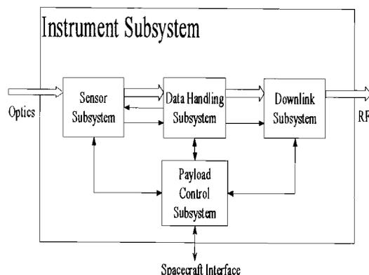
**Figure 4. Layout of ARIES Instrument Electronics**
