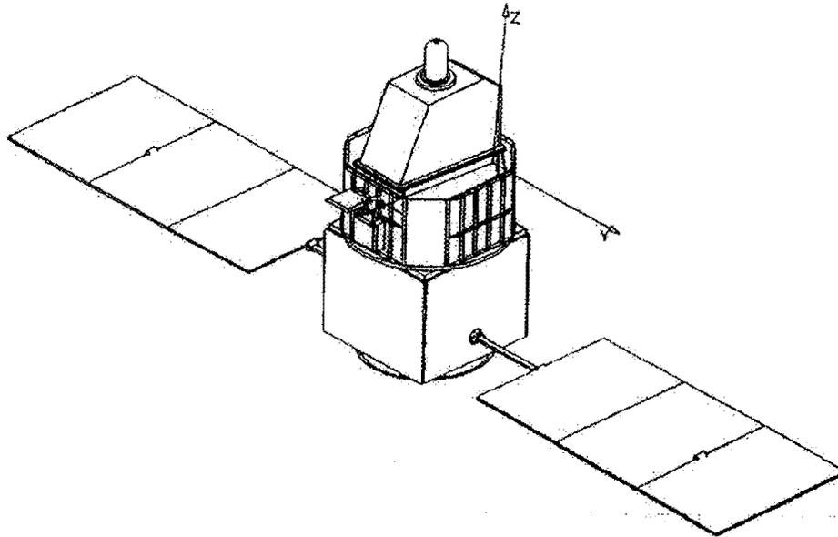
**Figure 2. ARIES Spacecraft in On-Orbit Configuration**
