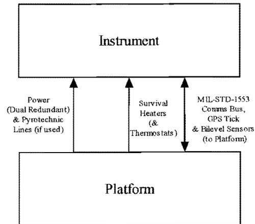
**Figure 1. Instrument and Platform Interfaces**
