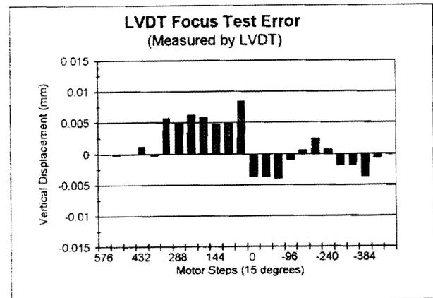
Figure 12 Focal plane focus error by LVDT
