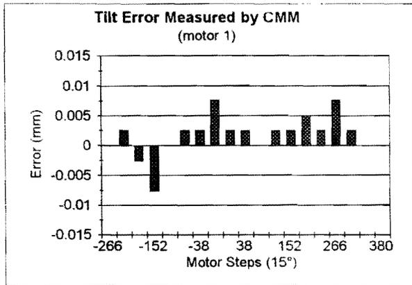
Figure 10 CMM measured difference in Motor 1
