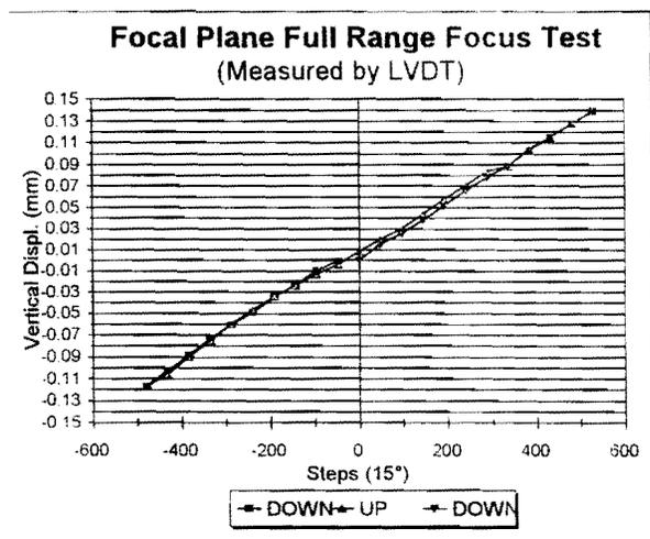
Figure 11 Simulated focal plane focussing results by the LVDT
