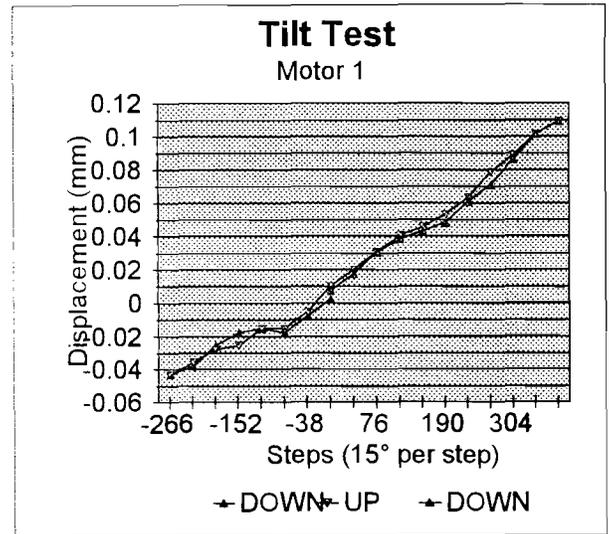
Figure 9 Tilt test results of Motor 1 by the CMM
