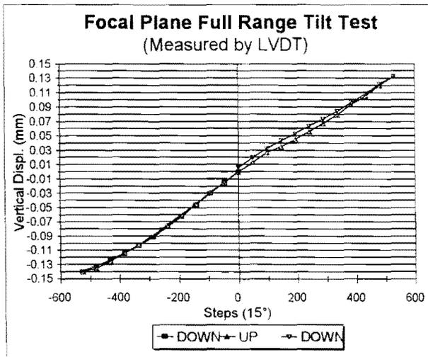
Figure 14 Motor 3 tilt performance as measured by the LVDT
