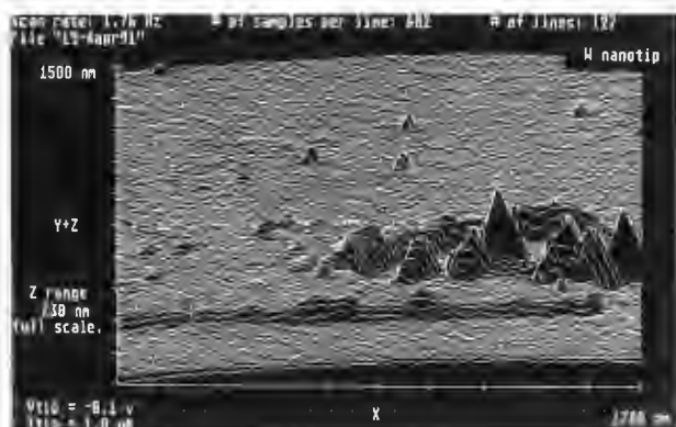
Fig.4. STM image of a carbon coated mH sheath which was damaged by previous imaging at a gap resistance of 100 MΩ. The carbon coating was \approx 4 nm thick.
