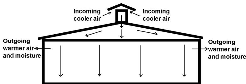
In small chicken houses, these factors can generally be sufficiently controlled without employing power ventilation (i.e. fans). The judicious and well-placed use of windows and vents will usually suffice. During summer, natural convection and/or gentle breezes will usually be adequate to drive air out the upper vents, or cupola, and bring in fresh air through windows or lower vent openings. Place upper vent openings on the side opposite of wind direction (i.e. leeward side).
