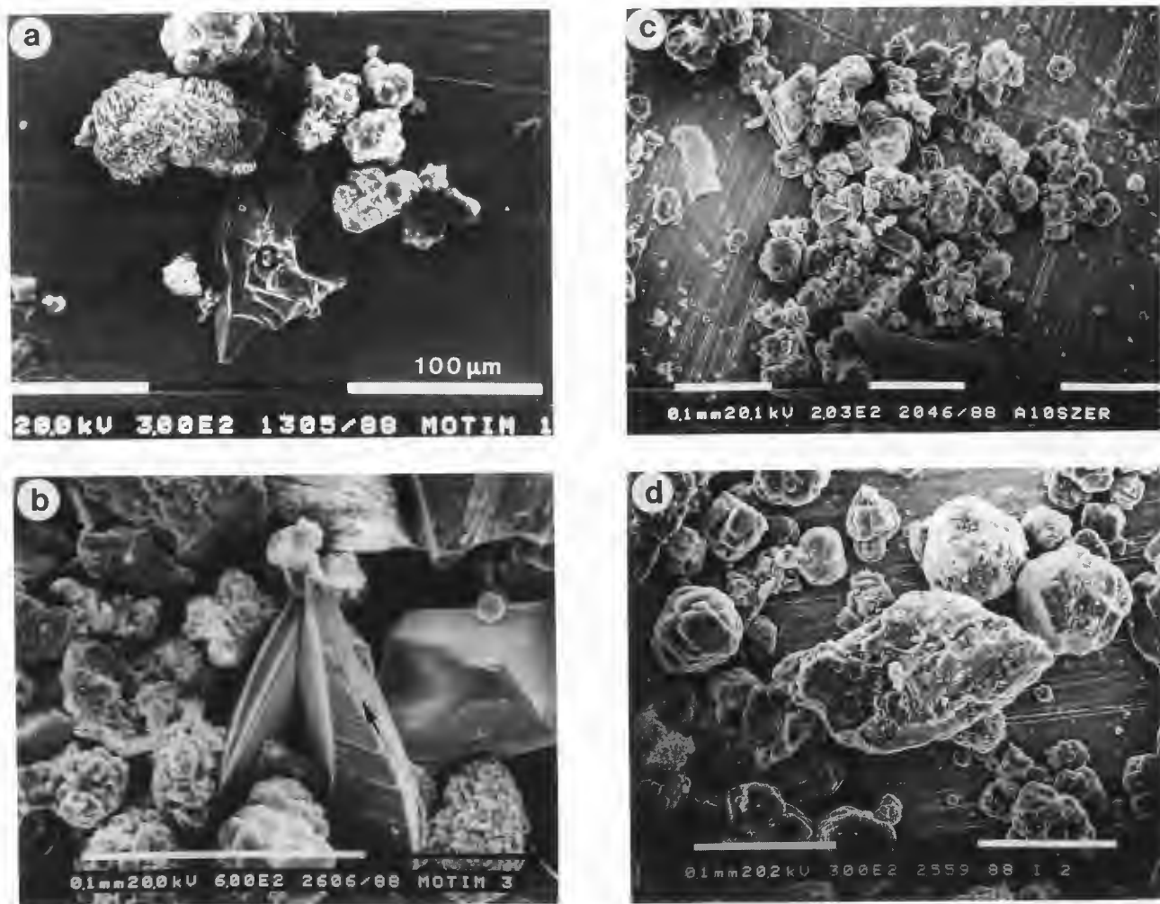
Figure 4: Secondary electron images of sedimentary particles collected at various places in Hungarian alumina plants and smelters.
