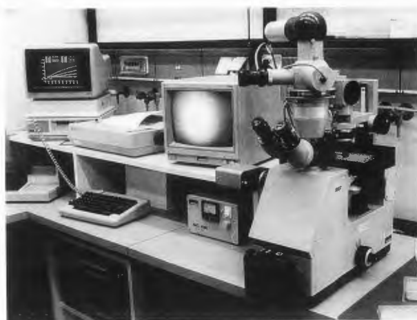
Figure 2: Computer controlled microphotometric system for multiple determinations of crystal growth rates in gel matrices (Gel Crystallization Method; GCM) comprising the following parts: Inverted microscope IM 35 with photometer and scanning stage adapted to microplates, stabilized power supply, electronic control unit, video camera (Carl Zeiss, W.-Germany) and computer HP 9816 S.
