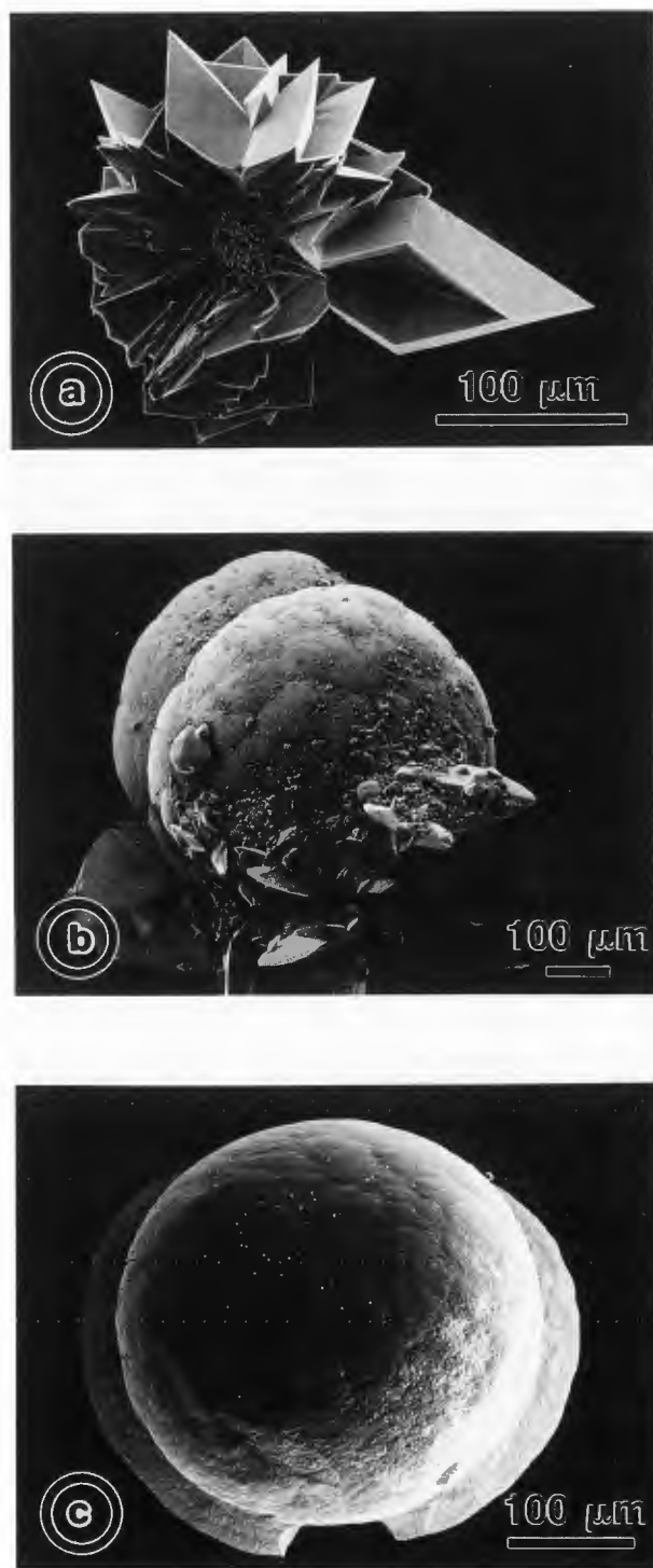
Figure 12. Different stages of phase transition of COD in the calcium chamber of the gel crystallization system after six weeks in the presence of mucin. The COD cluster (a) was transformed to COM by spherulization (b) and produced a smooth spherical crystal (c).
