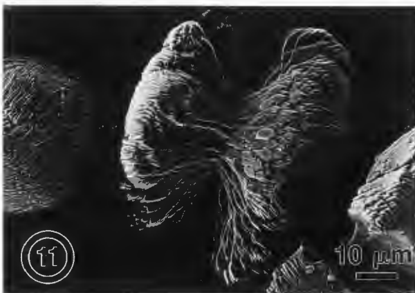
Figure 9. COD cluster grown in the calcium chamber of the gel crystallization system after two weeks in the absence of mucin.
