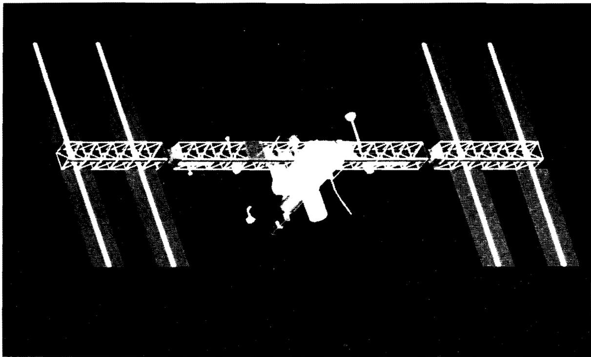
**Figure 8. Current Space Station Phase I Baseline Design. The Horizontal Truss Will Be Made From Graphite/Epoxy Struts to Which Laboratory and Habitation Modules and Solar Panels are Attached (NASA photo)**
