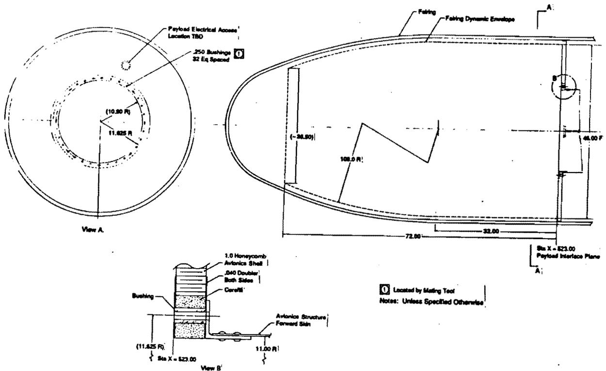
Figure 5 Pegasus Payload Volume and Mechanical Interfaces
