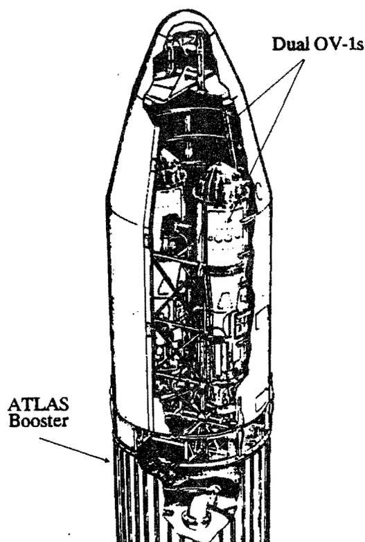
Figure 4. Dual OV-1s on an early Atlas booster.
