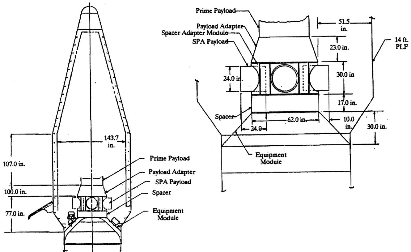
Figure 6. Spacer Adapter Concept for Centaur-Mounted SPA Payloads.
