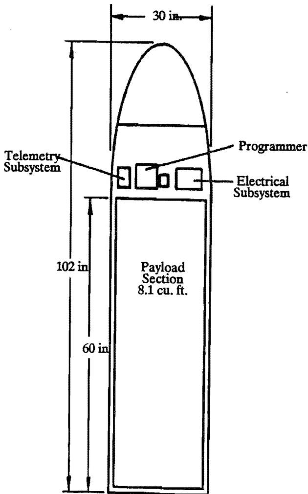
Figure 2. The Standard SPP Accommodated Canisterized Payloads.
