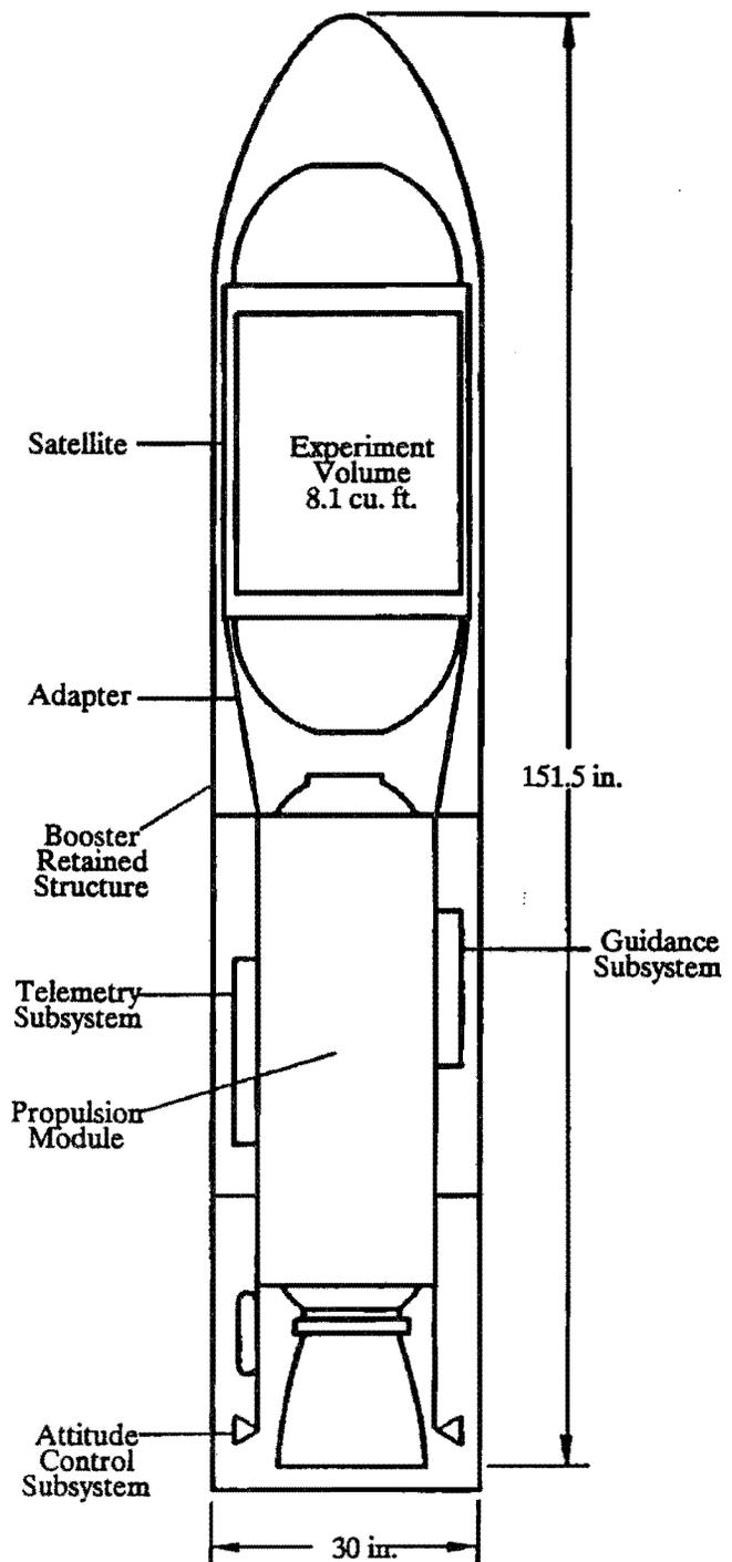
Figure 3. SPPs Also Supported Propulsive Payloads (GD's OV-1 Depicted).
