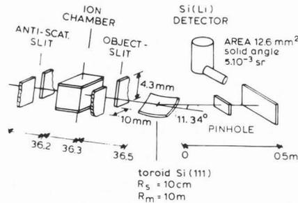
Fig. 7. Schematic layout of the set up used for the development of a synchrotron microprobe
