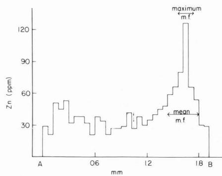
Fig. 5. Zn distribution obtained from the scan given in fig. 6. Shown is a typical result of a hippocampal section from a rat with a control diet of 50 mg Zn. The position of the mossy fibers is indicated. Frozen tissue was sectioned in 30  $\mu\text{m}$  slices, mounted and freeze-dried. Beam size was about 50  $\mu\text{m}$  and the beam current 0.1 nA.
