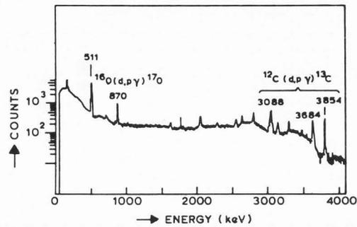
Fig. 3. Deuteron induced  $\gamma$ -ray spectrum used for measurement of C- and O-losses under bombardment.
