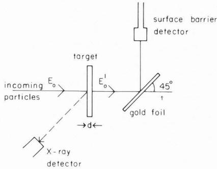
Fig. 1. Beam and target geometry used for concentration assignment.
