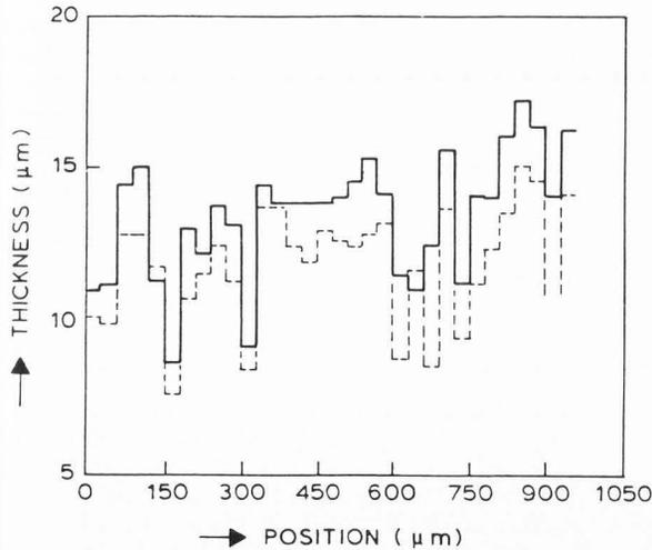
Fig. 2. Matrix thickness distribution of brain tissue before (solid line) and after (dotted line) proton bombardment for 1 hr with 1 nA beam. Results shown are from a line scan divided into 32 pixels.
