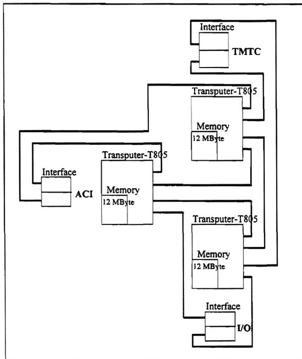
Fig. 4: Onboard Computer Architecture.
