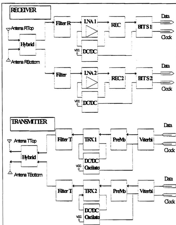
Fig. 5: Communication Subsystem Diagram.
