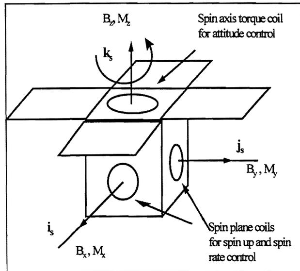
Fig. 3: Torque coils configuration on the satellite.
