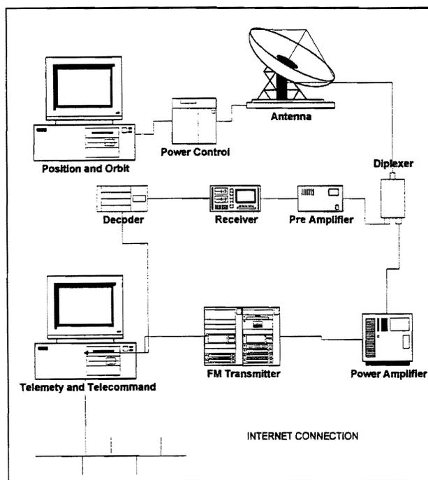
Fig. 6: Ground Station Block Diagram.
