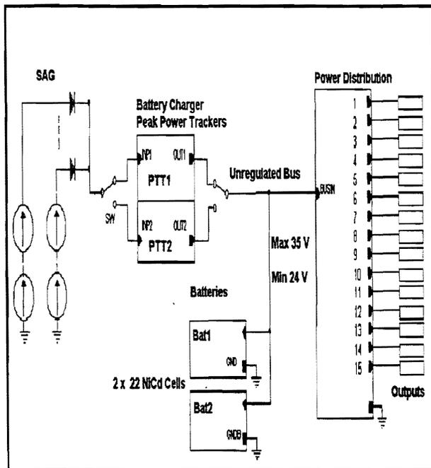
Fig. 2: Power Supply Subsystem Block Diagram.
