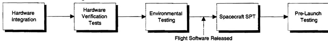
I&T Flow After Final Flight Software Release
