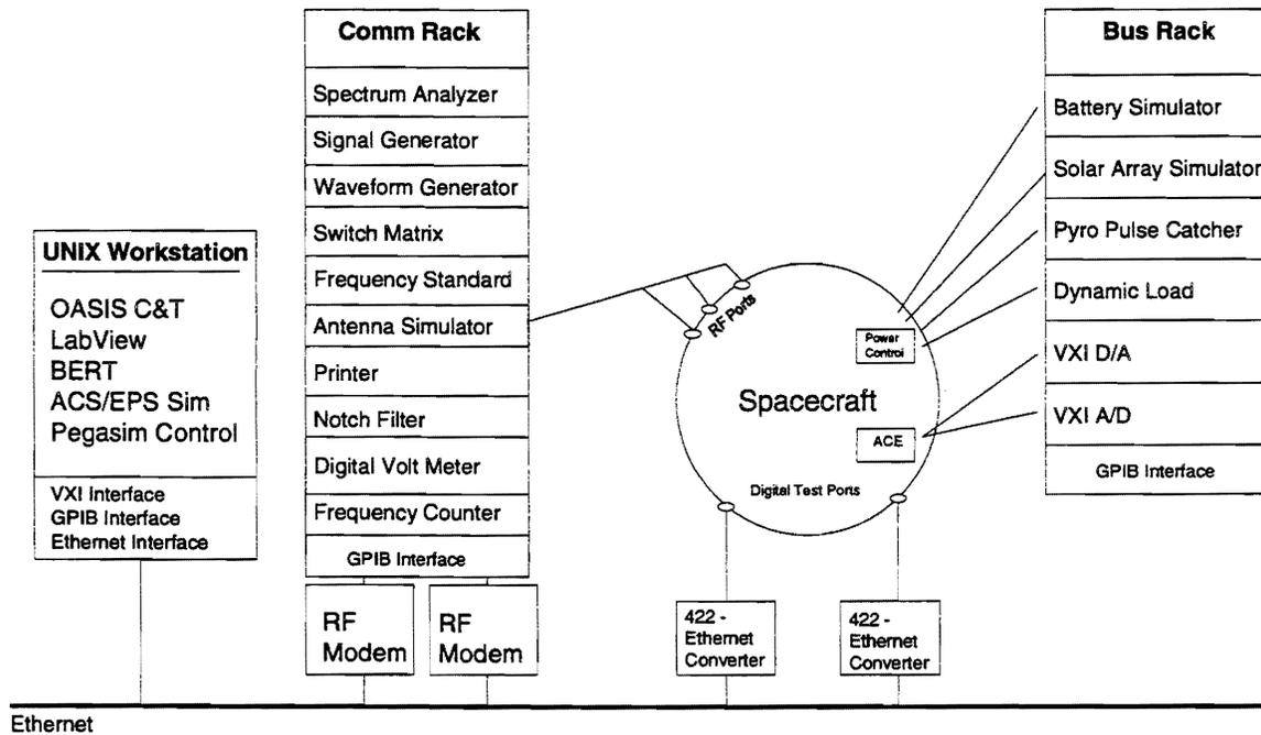
Figure 3 Spacecraft Test Equipment
