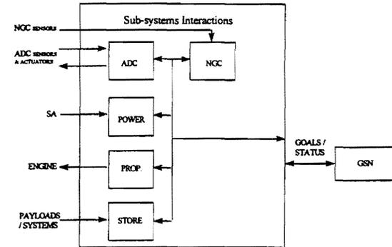
**Figure 4-4 Spacecraft sub-system interaction**
