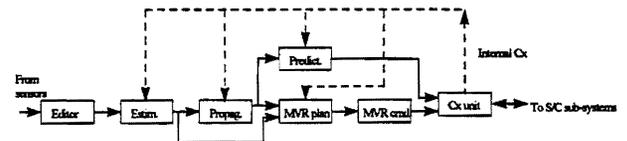
Figure 4-1 Autonomous navigation system
