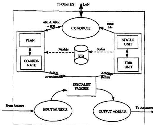
**Figure 4-3 Generic autonomous sub-system**
