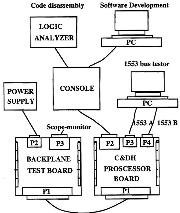
Figure 2. Test setup.
