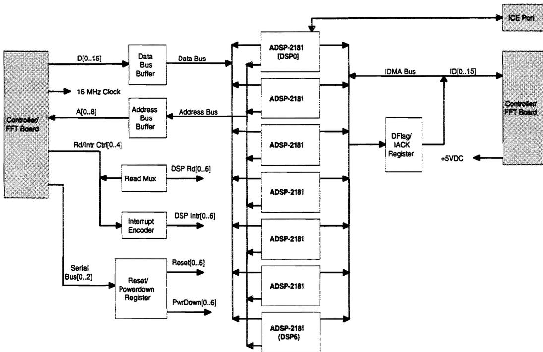
Figure 3. Receiver Digital Section.
