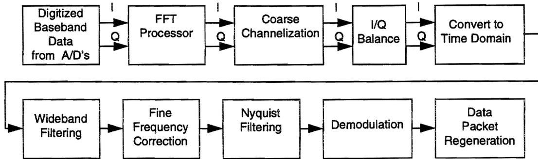
Figure 4. DSP Software Algorithm Flow.
