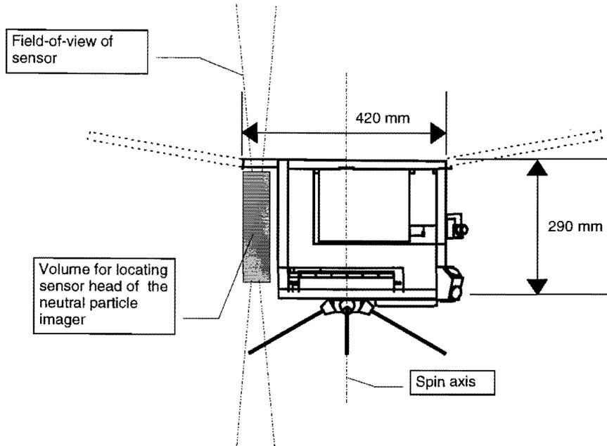
**Figure 2** The location of ASTRID's main instrument.
