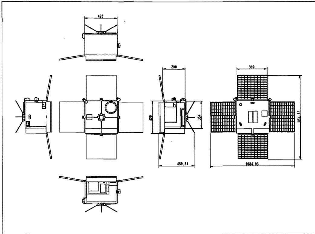
Figure 4 Dimensions of the ASTRID microsatellite
