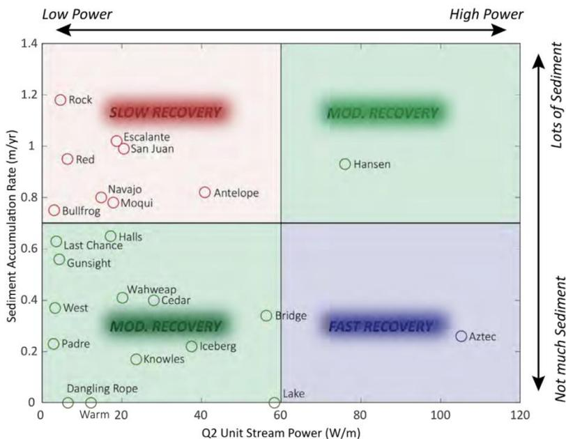
**Figure 3.** This scatter plot from Kasprak & Schmidt (2019) shows the unit stream power of 23 tributaries in Lake Powell compared to the average annual sediment accumulation rate for those streams from 1959 to 2017.
