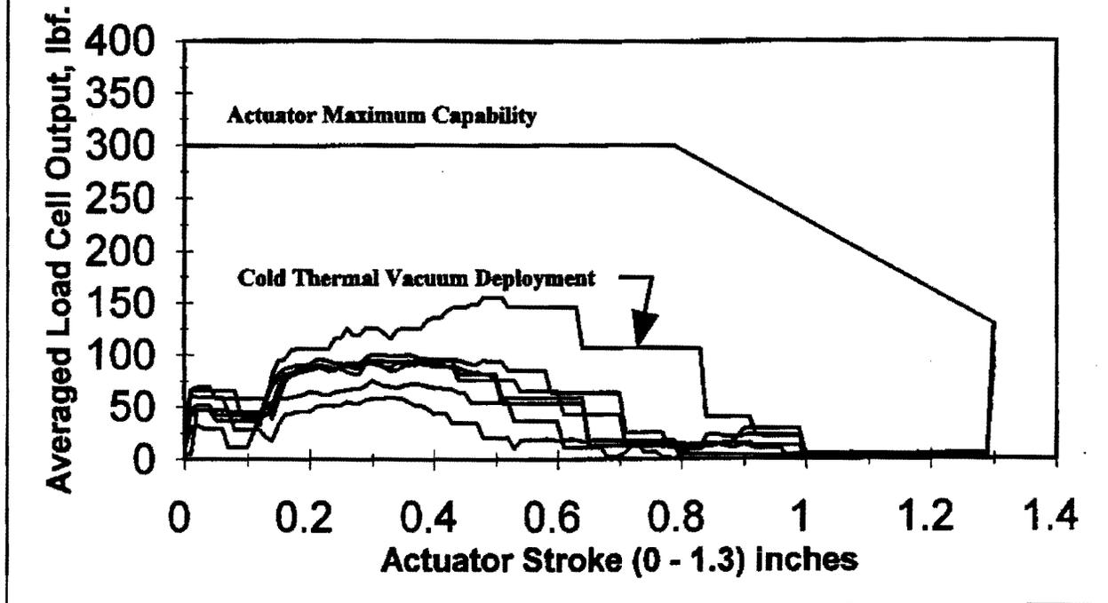
Figure 8, Composite Solar Array Deployments (-X Wing)
