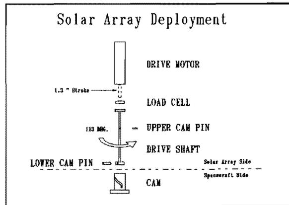
**Figure 4, Mechanism Components**
