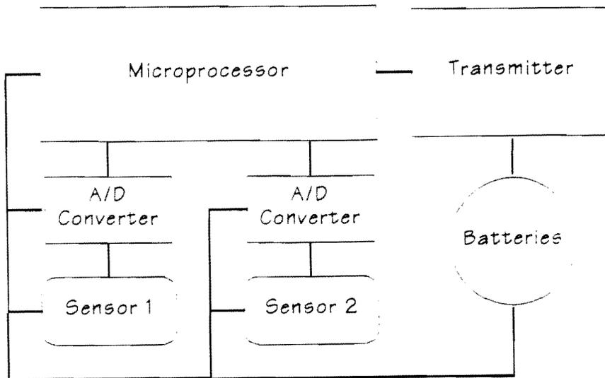
**Figure 3 - PicoSat Functional Schematic**
