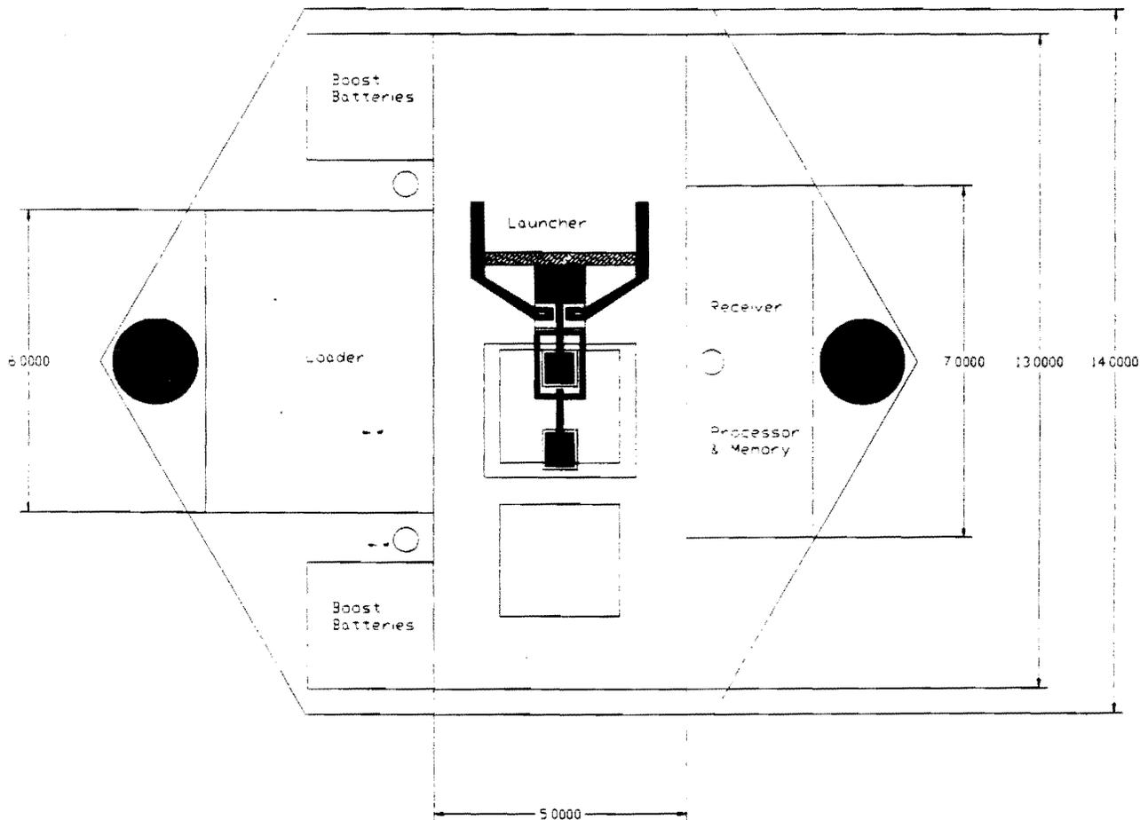
**Figure 4 - Layout of the PicoSat tray**
