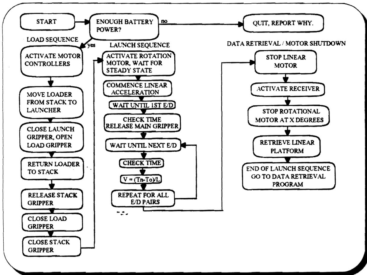
Figure 6 - PicoSat Load/Launch Sequence
