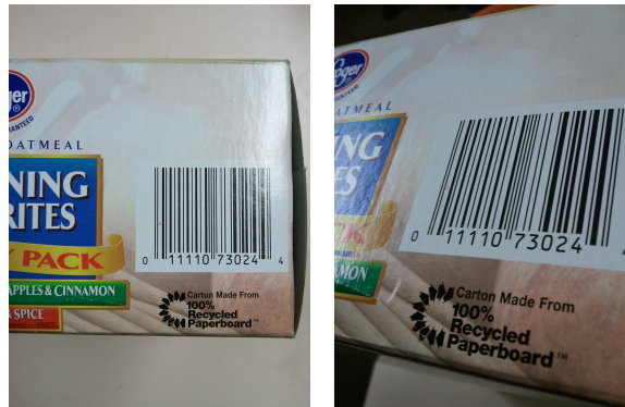
Figure 3.4. Examples of image (left) and its skew distorted equivalent (right).
