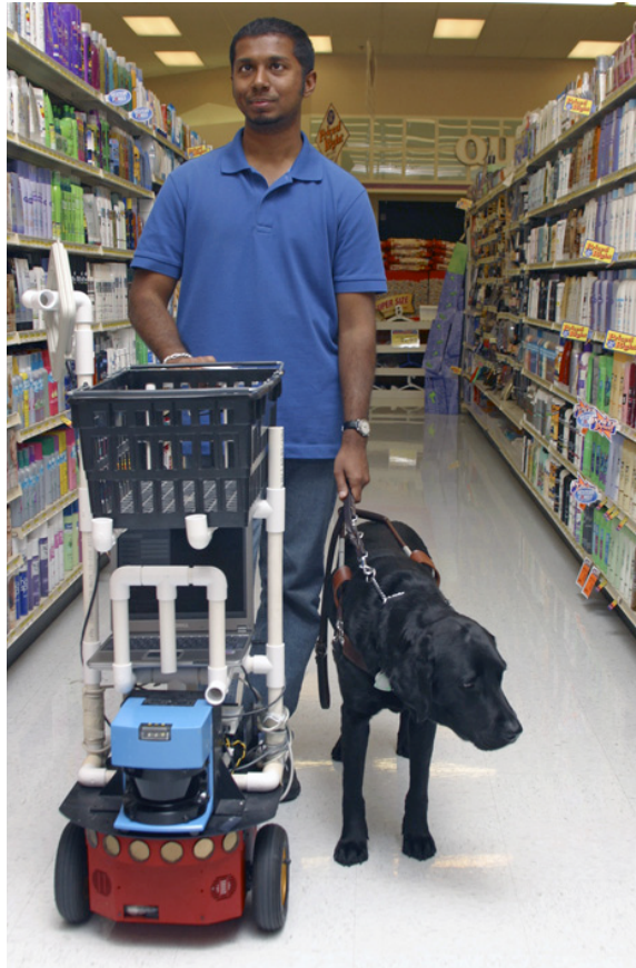
Figure 2.1. RoboCart assistive shopping system.
