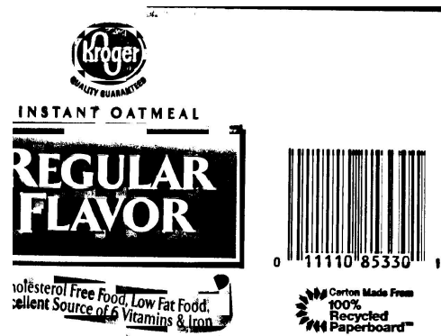
(d) Binarized image obtained using our modified Niblack method
