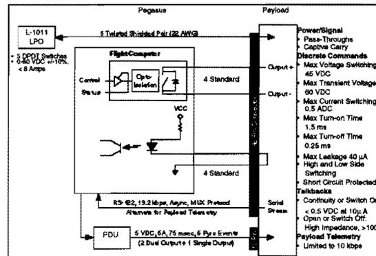
Figure 6. Pegasus Payload Electrical Interface
