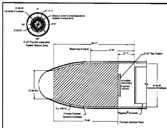
Figure 3. Payload Fairing Dynamic Envelope with 23 Inch Diameter Payload Interface
