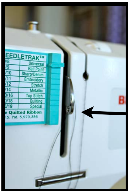
Figure 9. Thread take-up lever.
