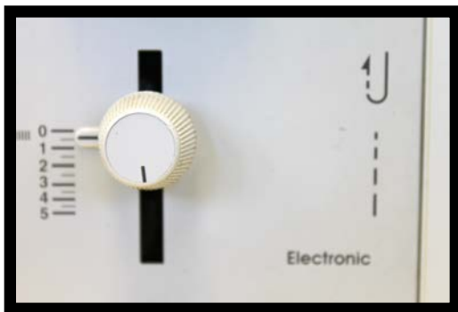
Figure 15. Stitch length selector.
