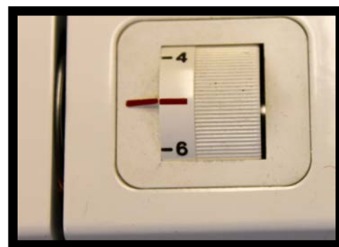
Figure 13. Thread tension selector.
