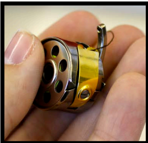
Figure 3. Threaded bobbin inserted into bobbin case.
