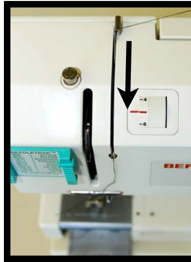
Figure 7. First thread guide on top of sewing machine.
