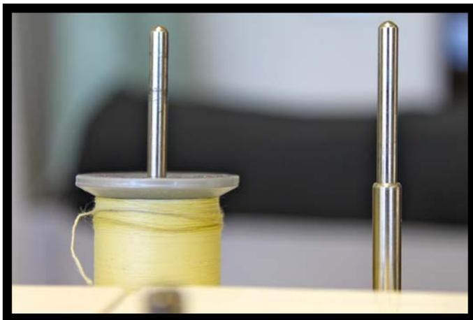
Figure 6. Thread on spool pin.
