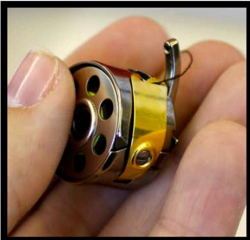
Figure 3. Threaded bobbin inserted into bobbin case.
