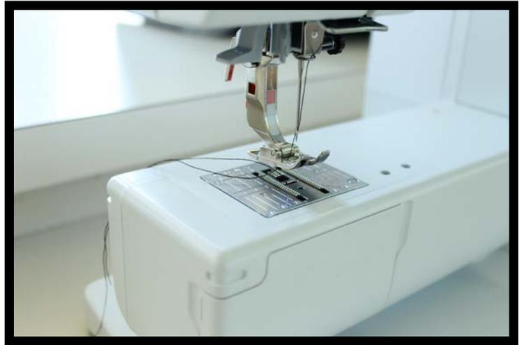
Figure 12. Threaded sewing machine.
