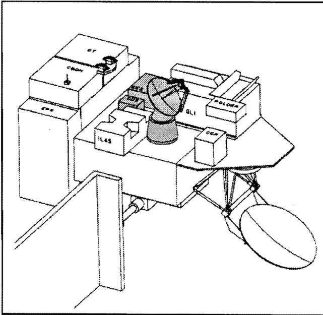
**Figure 4. The SeaWinds backscatter radar wind vector sensor**
