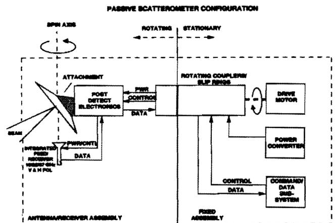
**Figure 2. Integrated feed/receiver simplifies instrument design**
