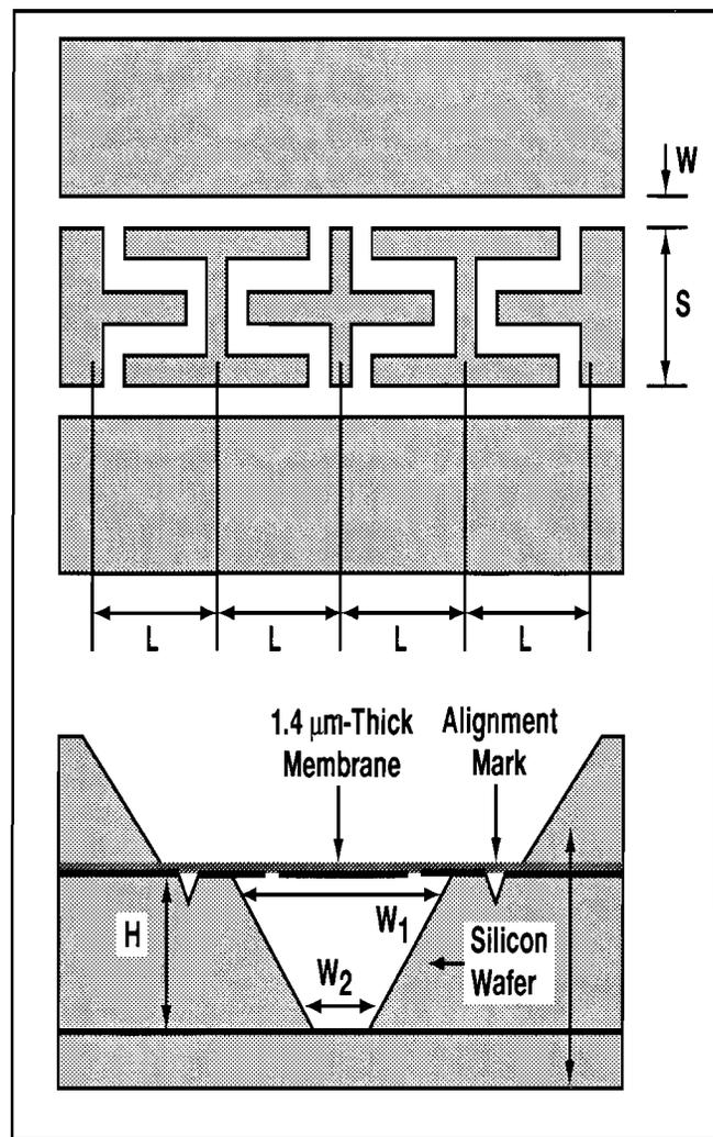
**Figure 3. Micromachined Filters**
